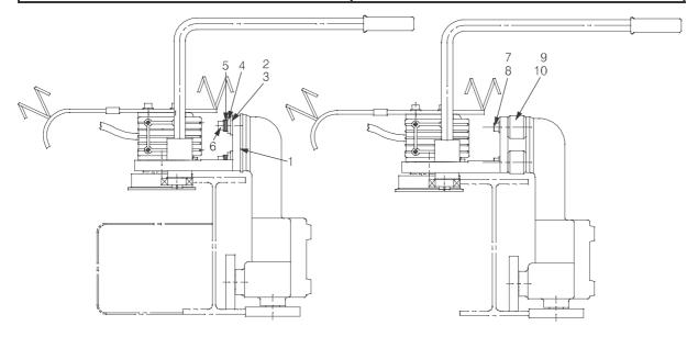
When an unmachined beam is to be used the positions 1-6 (fitted on delivery) are to be replaced by the supplied positions 7-10 (four of each).
