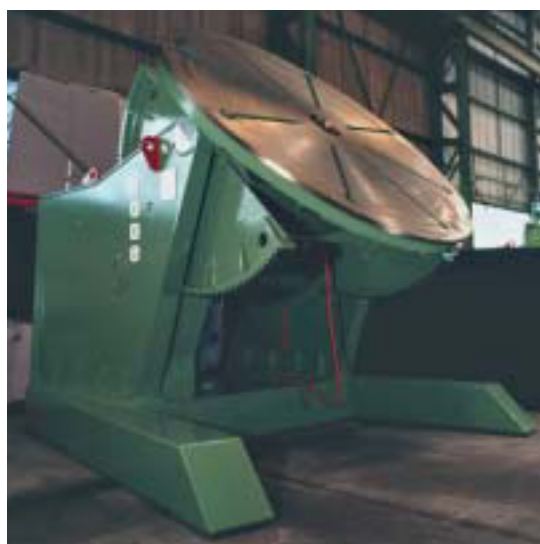
Model VP.25 Positioner (Capacity 25,000 kgs)
